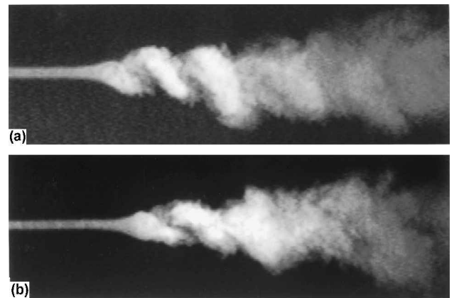
Fig. 4 Conical/spiral vortex breakdowns at Re = 1.2 \times 10^5 . The exposure time = 6 ns (scale: 5 mm in figure = 1 mm in reality).
